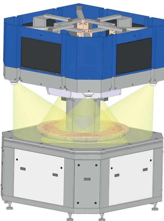
Video cameras can be oriented in any angular position to look inside the machine only or in other critical location of the machine. The recorder linked to the PLC can store up to 15 days of continuous video at 60ips. Once the disk is full the new records overwrite the oldest one.
